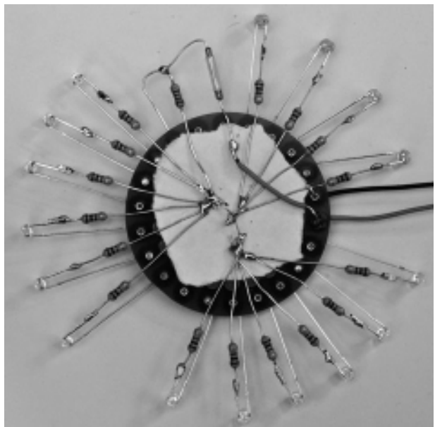
Figure 9-14 Bottom side of Lilypad board.
